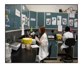
\*\* Equipment: The VDCI Surveillance Laboratories are fully equipped with 8 stereo zoom binocular microscopes, including one video/photographic microscope capable of projecting microscopic images onto computer screens or to projection equipment for wall sized viewing.
